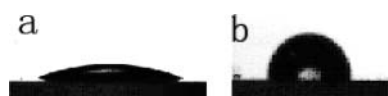
Fig. 1 Water counteranion (CA) of glass: (a) pure glass, CA < 10°, (b) glass coated with the SAM of [C 16 tespim]Br, CA = 98±2°.
